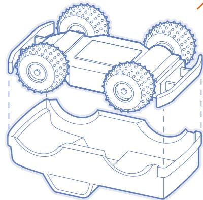
**2** Turn the truck over and remove the screws that hold the truck body to the chassis. Carefully lift the body off, pulling the antenna wire through the hole. Leave the front bumper/winch assembly on the front to provide extra stability for front-end bumping. Save the body parts and screws.
