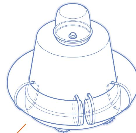
**6** Add the foam noodle around the opening of the robot's body to act as a bumper. Trim the noodle to fit, then use an awl or drill to make holes at the back and front as shown in the diagram. Attach the noodle to the body using nylon wire ties.
