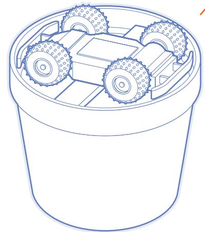
**3** Center the 1-by-2-inch wood block and chassis, wheels up, on the plastic tub. Slide the chassis forward so the front bumper touches the tub. Mark and cut the block so it fits snugly inside—trim or sand the corners for a tighter fit. Glue the block to the flat part in the center of the chassis, above the motor battery compartment. Don't let glue get on the other parts of the chassis. Check the fit inside the plastic body and set aside to dry.
