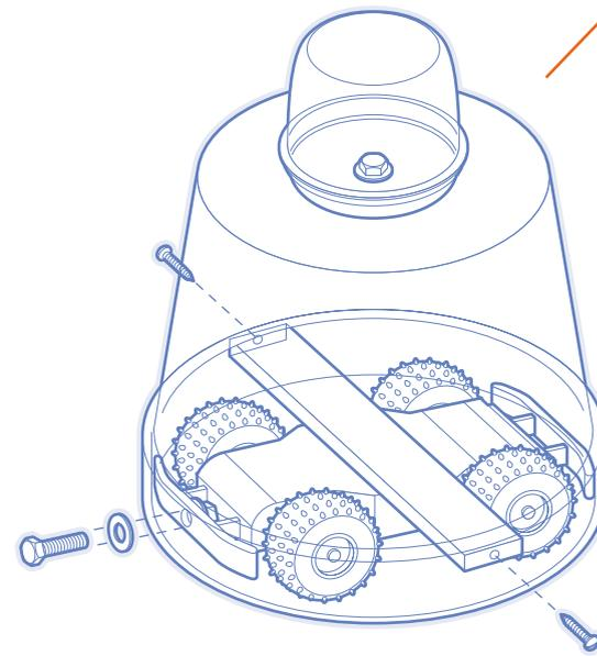
**5** Use an awl or drill to make a hole to attach the tub to the front bumper of the truck chassis. Secure with a bolt, nut and two flat washers. Mount the robot's plastic body to the chassis's wooden block with small wood screws. Make sure there is enough clearance for the wheels to turn and move freely. Tape the antenna wire to the inside of the body.
