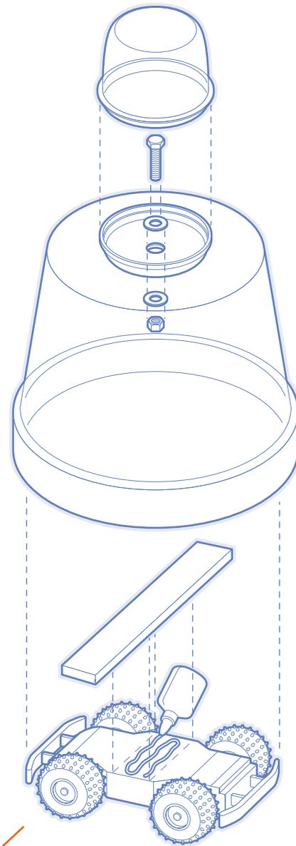
**4** Center the food storage container's lid on the bottom of the plastic tub. Use an awl or drill to make a hole through both. Attach the lid with a nut, bolt and two flat washers.
